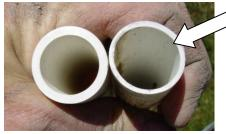
You don't need Sch. 40 pipe; the thinner PVC pipe can be used. This keeps the weight down and is easier to cut. ½" diameter
