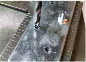
Next I made a template to find the center of the plugs, used it to mark all the plugs, and drilled a hole in the center of each.
