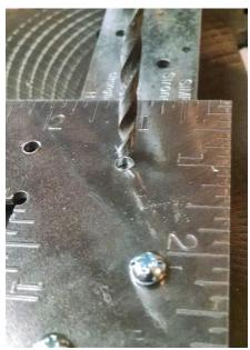
Once the strap is fully attached, flip the framing square over and drill through the strap using the hole you drilled for the pole as your guide.
