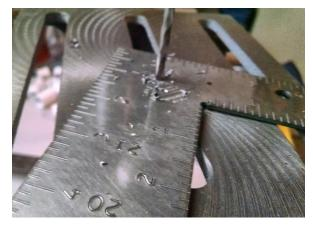
Drill the holes for each pole at the marks you made through the template.
